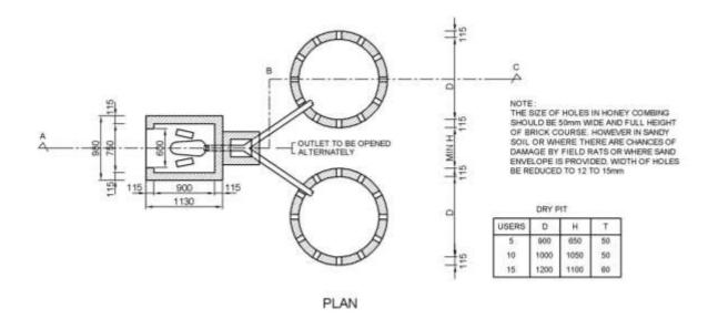
Figure 3: Pour-flush latrine in water-logged areas
