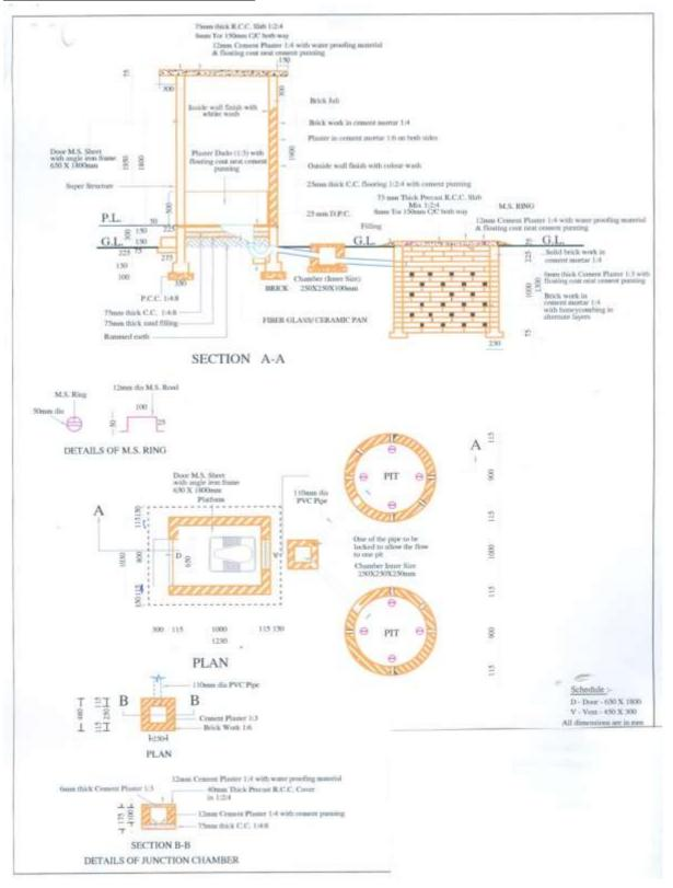
Figure 2: Pour-flush latrine with circular pits
