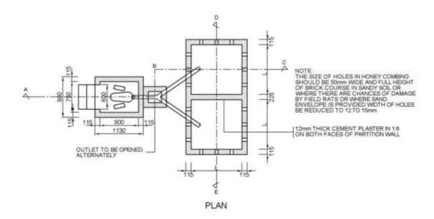
Figure 6: Typical sketch of two-compartment septic tank for 5 users
