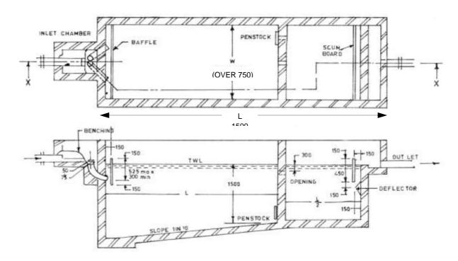
Figure 7: Details of bio-digester with reed bed
