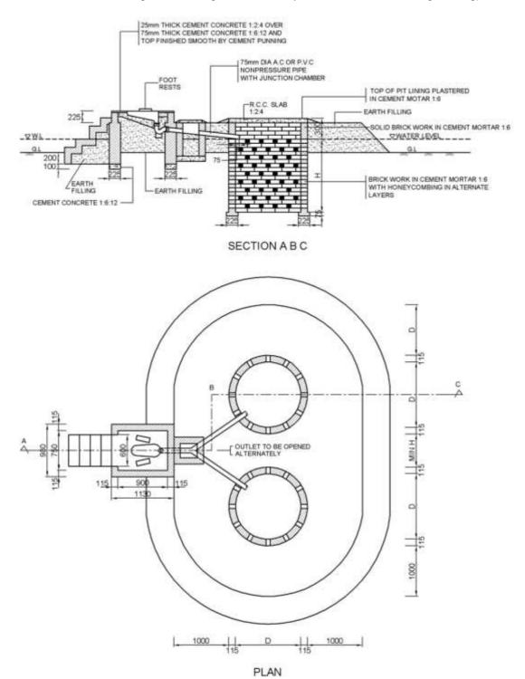
Figure 4: Leach pits in high subsoil water level
