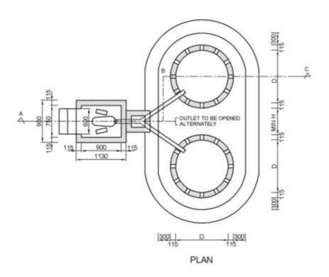
Figure 5: Pour-flush latrine with combined pits
